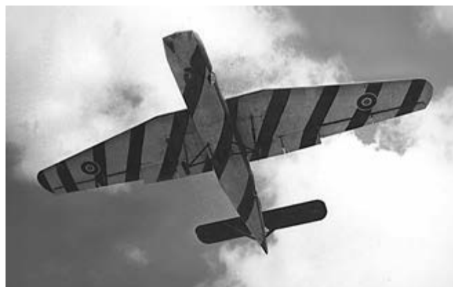
Above: An Airspeed Horsa glider returning from a training flight from North Luffenham, clearly showing the underside yellow and black striping (Airfield Focus)
